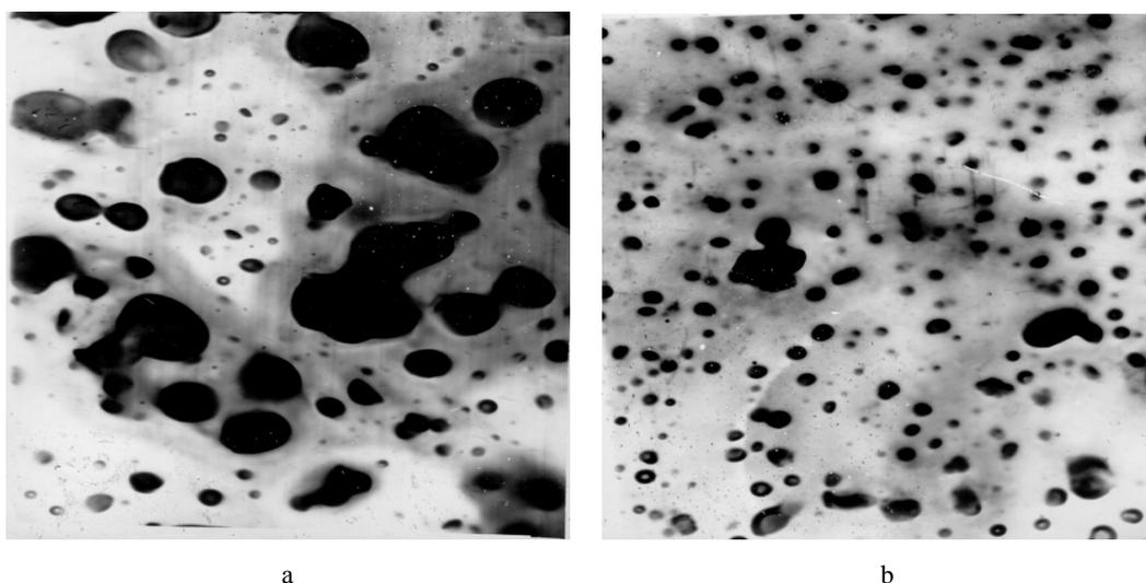
**Fig. 4.** Results of electron microscopic study of buckwheat husk briquette adsorbent (6700 times increased) at different stages of its production: a – raw material grinding and interaction with sulphate acid; b – mechanical and chemical activation
