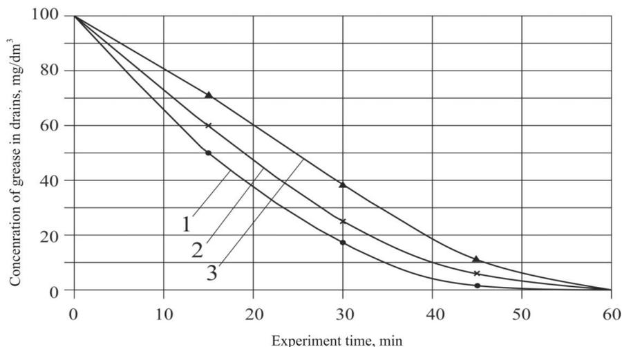
**Fig. 6.** Dynamics of changes in the time of concentration of technological grease in contaminated water with the use of adsorbent of different granulometric composition (mm): 1 – 0,03–0,01 mm; 2 – 0.1–1.0; 3 – 1.0–3.0
