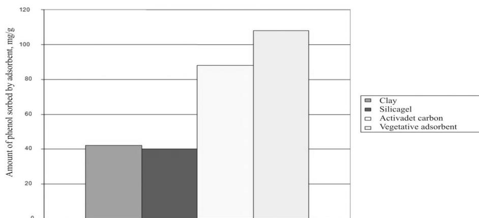
**Fig. 5.** Results of absorption of phenol by various adsorbents
