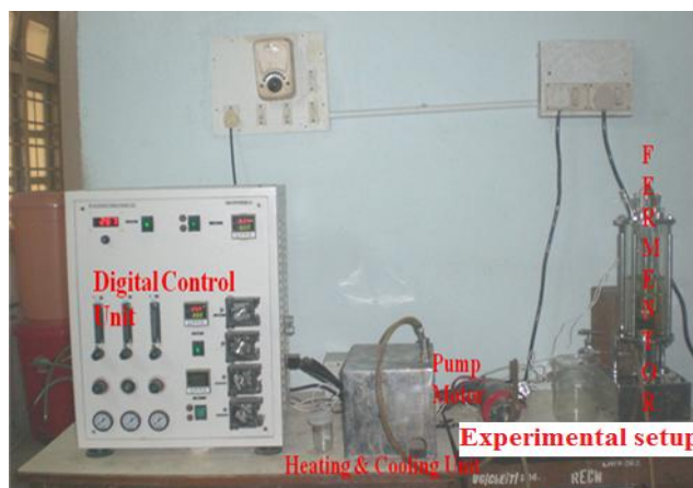
Fig. 1. Batch fermentation set-up
