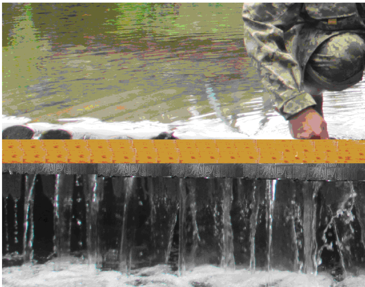
Fig. 3. A bioreactor-type structure based on a fibrous carrier “Viia” and wooden structures – “casings”
