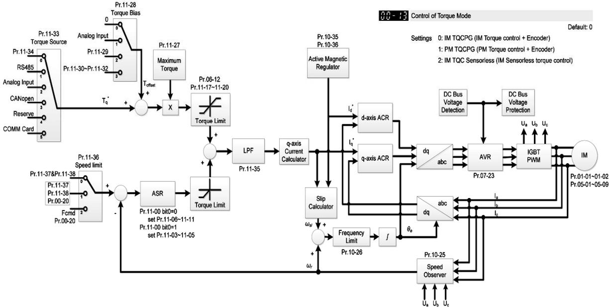
Fig.1. Induction motor in sensorless torque control mode for Delta C2000 VFD.
