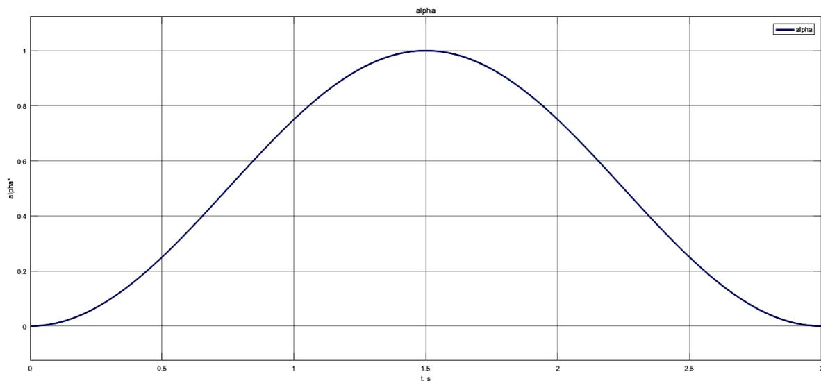
Fig. 3 Rope deviation angle
