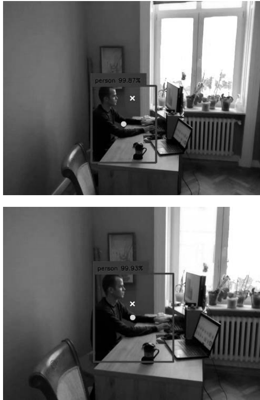
Fig. 10. Example of recognition and tracking modules work on mobile system. The big white cross represents the center of the screen, white dot – a center of the recognized object
