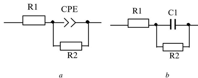
Fig. 1. Electrode-electrolyte system substitution schemes (aqueous NaCl salt solution) for frequencies not exceeding 1 kHz: C1 is the double electric layer capacitance, CPE is the constant phase element, R1 is the electrolyte resistance, R2 is the interphase transition resistance
