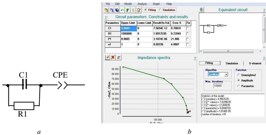
Fig. 8. Modeling of the electrochemical system of aqueous sugar solution: *a* – the substitution scheme of the electrode – non-electrolyte system for aqueous sugar solution); *b* – the impedance spectrum of the sugar solution
