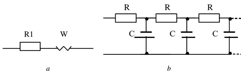
Fig. 6. Warburg impedance: a – the substitution scheme of the electrode-electrolyte system, taking into account the impedance of Warburg; b – and the equivalent Warburg impedance scheme
