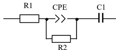
Fig. 5. Substitution scheme of the electrode-electrolyte system, taking into account the electrode capacity  $C1$
