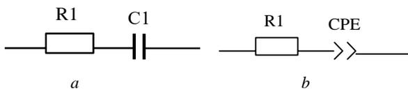
Fig. 3. Substitution scheme of the electrode-electrolyte system: a – for a perfectly polarized electrode, on which no electrochemical reaction occurs; b – in the presence of diffusion phenomena in the electrode region and the flow of Faraday current due to electrode reactions
