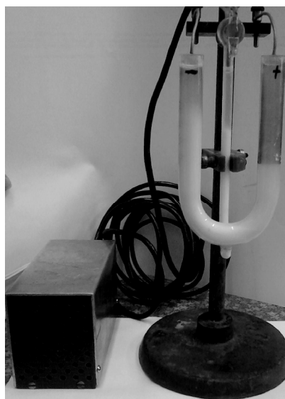
Fig. 2. Electrophoresis of \text{Ca}(\text{OH})_2 suspension with Burton’s apparatus
