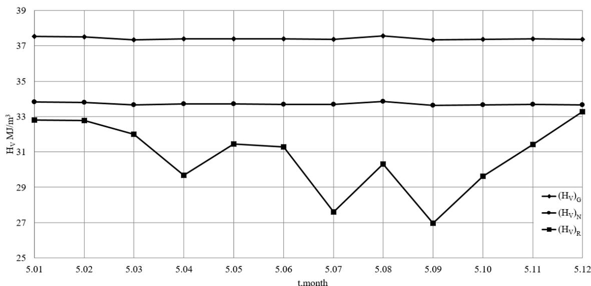
Figure. Change in the calorific value of natural gas during the year on the 5th day of each month
