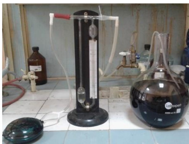
Fig. 2. Scheme of an experimental plant for studying the efficiency of biological aerobic treatment of the landfill filtrate in aeration conditions
