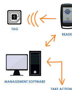
Fig. 1. Basic components of the RFID system.
