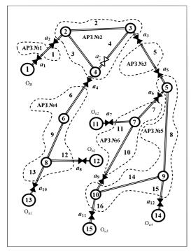
Fig. 1. Chart of dividing the original graph of the pipeline transport network into subgraphs of emergency repair zones.
