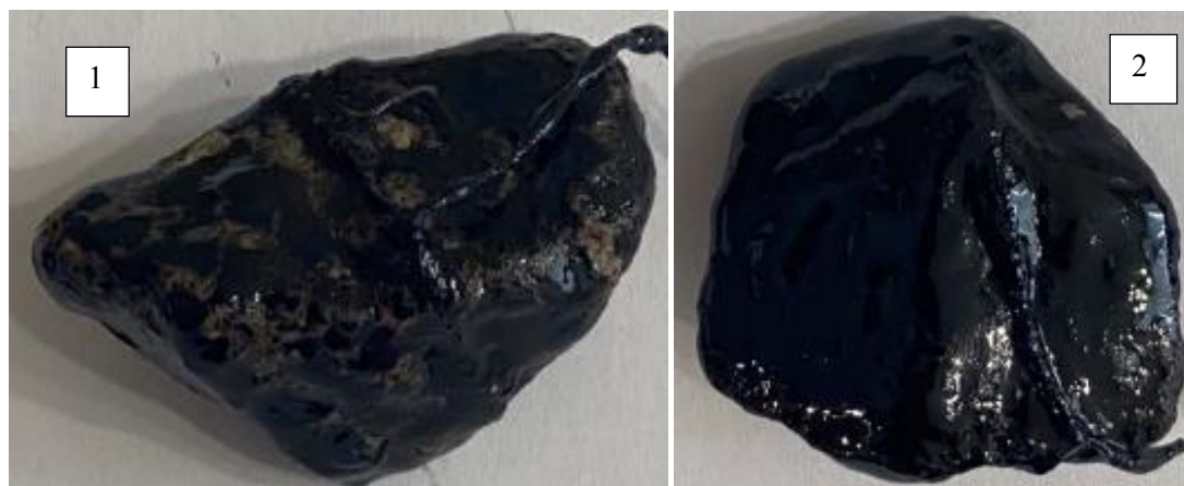
Fig. Adhesion to gravel: 1 – 100/150 (2 points), 2 – BMW 60/90 (5 points).
