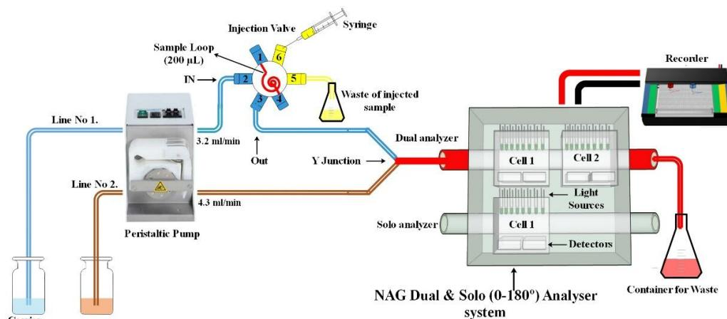
Fig. 4. A diagram shows the flow manifold system used in the determination of MBH
