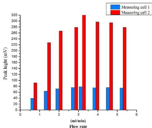
**Fig. 9.** The effect of flow rates on the height of peaks using initial conditions: MBH 7  $\mu\text{mol/L}$ , sodium persulfate 60  $\mu\text{mol/L}$ , open valve mode and 200  $\mu\text{L}$  sample volume
