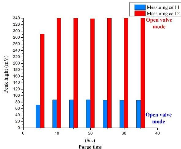
**Fig. 11.** The effect of the purge time the height of peak using initial conditions: MBH 7  $\mu\text{mol/L}$ , sodium persulfate 60  $\mu\text{mol/L}$ , flow rates 3.3 & 4.3  $\text{mL min}^{-1}$  for distilled water and sodium persulfate (reagent) lines, respectively, and 250  $\mu\text{L}$  sample volume
