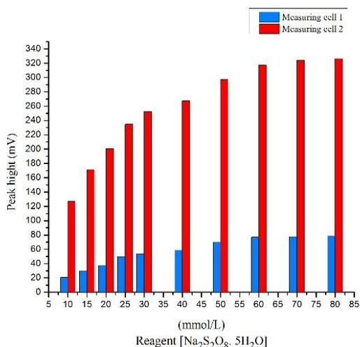
**Fig. 6.** The effect of sodium persulfate concentrations on the height of peaks using initial conditions: MBH 7  $\mu\text{mol/L}$ , flow rates 2.8 & 3.2  $\text{mL min}^{-1}$  for water and reagent lines, respectively, open valve mode and 200  $\mu\text{L}$  sample volume
