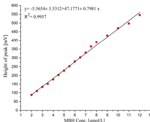
**Fig. 13.** The linear calibration curve for determination of MBH for measuring cell 2 using all of the optimum conditions: sodium persulfate 60  $\mu\text{mol/L}$ , flow rates 3.3 & 4.3  $\text{mL min}^{-1}$  for distilled water and sodium persulfate (reagent) lines, respectively, open valve mode and 250  $\mu\text{L}$  sample volume
