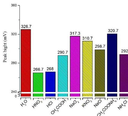
**Fig. 8.** The effect of using different aqueous mediums on the height of peaks for measuring cell 2 using initial conditions: MBH 7  $\mu\text{mol/L}$ , sodium persulfate 60  $\mu\text{mol/L}$ , flow rates 2.8 & 3.2  $\text{mL min}^{-1}$  for water and reagent lines, respectively, open valve mode and 200  $\mu\text{L}$  sample volume. Note: all of the used aqueous solutions were used instead of distilled water in this experiment
