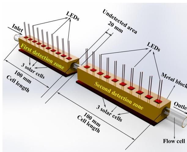
**Fig. 3.** A diagram shows the major components of the NAG Dual & Solo (0–180°) analyzer
