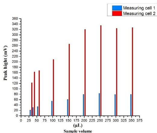
**Fig. 10.** The effect of using variable volumes of sample of the MBH on the height of peak using initial conditions: MBH 7  $\mu\text{mol/L}$ , sodium persulfate 60  $\mu\text{mol/L}$ , flow rates 3.3 & 4.3  $\text{mL min}^{-1}$  for distilled water and sodium persulfate (reagent) lines, respectively, and open valve mode
