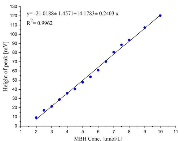
**Fig. 12.** The linear calibration curve for determination of MBH for measuring cell 1 using all of the optimum conditions: sodium persulfate 60  $\mu\text{mol/L}$ , flow rates 3.3 & 4.3  $\text{mL min}^{-1}$  for distilled water and sodium persulfate (reagent) lines, respectively, open valve mode and 250  $\mu\text{L}$  sample volume
