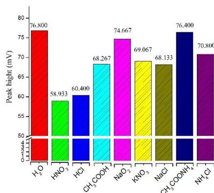
**Fig. 7.** The effect of using different aqueous mediums on the height of peaks for measuring cell 1 using initial conditions: MBH 7  $\mu\text{mol/L}$ , sodium persulfate 60  $\mu\text{mol/L}$ , flow rates 2.8 & 3.2  $\text{mL min}^{-1}$  for water and reagent lines, respectively, open valve mode and 200  $\mu\text{L}$  sample volume. Note: all of the used aqueous solutions were used instead of distilled water in this experiment
