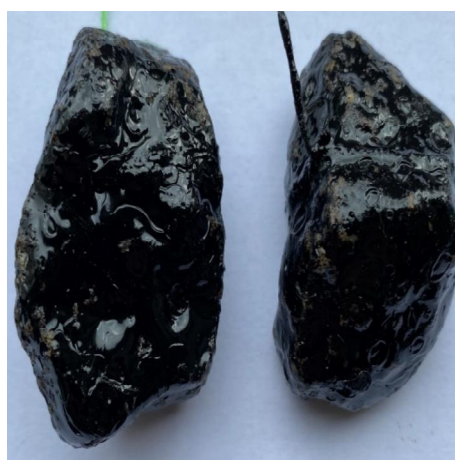
Fig. 6. Adhesion to CS-1 (a, b) and CS2 (c, d) of unmodified BO-1 (a, c) and modified BOMA-10 (b, d)
