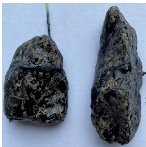
Fig. 6. Adhesion to CS-1 (a, b) and CS2 (c, d) of unmodified BO-1 (a, c) and modified BOMA-10 (b, d)
