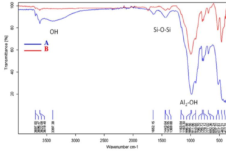
Fig. 1. FT-IR spectra of raw-Kaol (A) and Kaol-H<sup>+</sup> (B)
