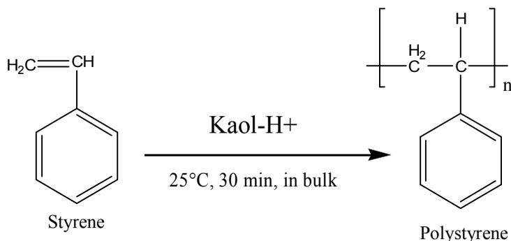
**Scheme 1.** Polymerization of styrene catalyzed by Kaol-H<sup>+</sup>
