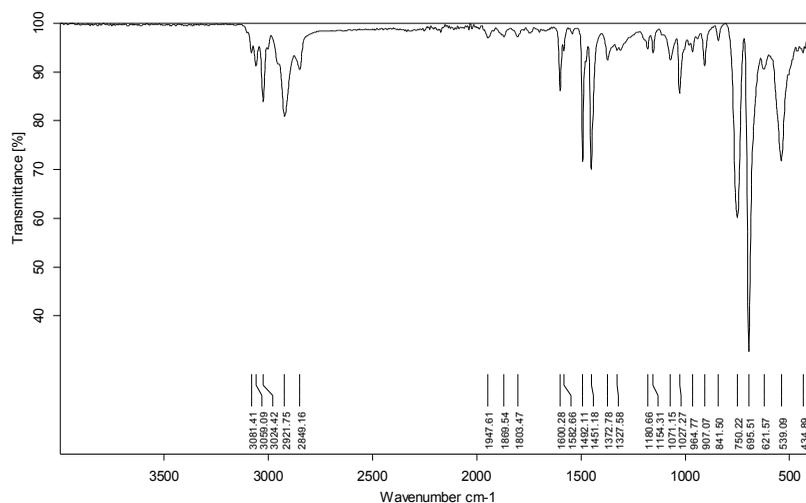
**Fig. 4.** FT-IR spectrum of the obtained polystyrene
