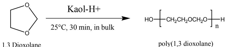
**Scheme 2.** Polymerization of 1,3-dioxolane catalyzed by Kaol-H<sup>+</sup>
