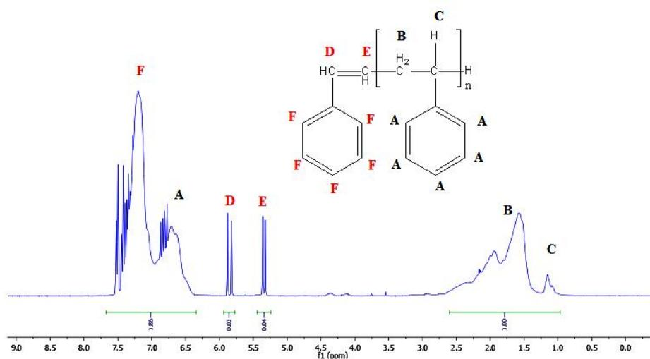
Fig. 6.  $^1\text{H}$  NMR spectrum of the obtained polystyrene
