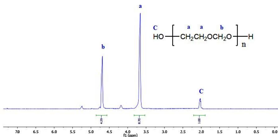
Fig. 7.  $^1\text{H}$  NMR spectrum of the obtained poly(1,3-dioxolane)
