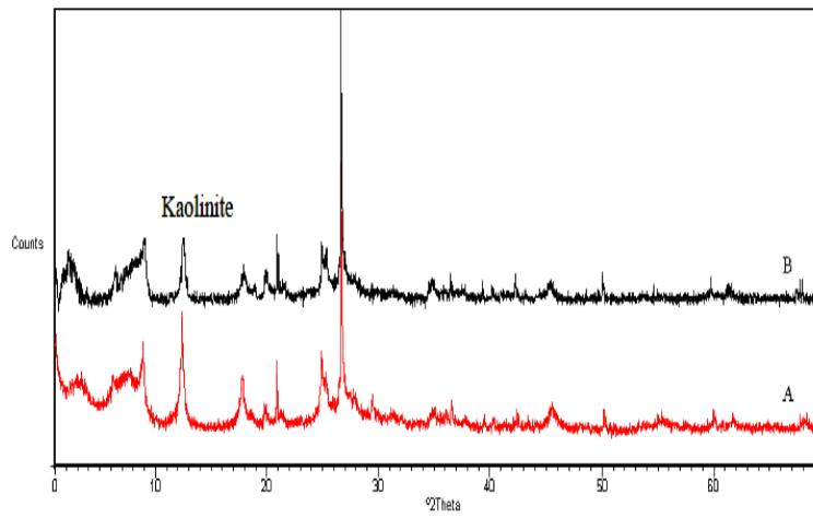
Fig. 2. X-ray diffractograms of raw-Kaol (B) and Kaol-H<sup>+</sup> 0.25M (A)
