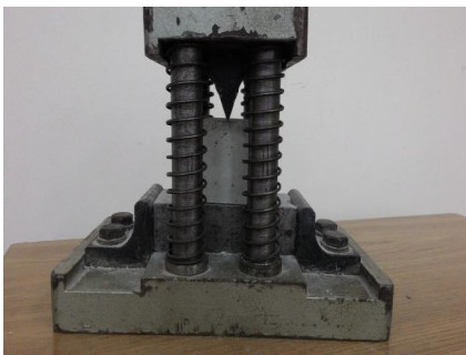
Fig. 2. Cell for determining the compressive strength under wedging
