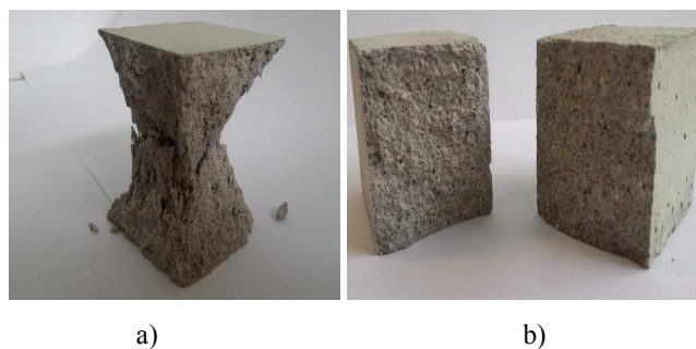
Fig. 1. Appearance of test beams after compressive test (a) and after flexural test (b)
