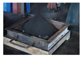
Fig. 1. Conditioned used molding mixture
