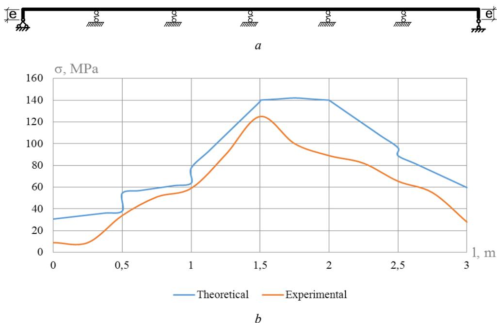
Fig. 7 Graph of stress distribution: a – calculation model of the stiffening girder, b – plot of normal stresses in the middle lines of the stiffening girder
