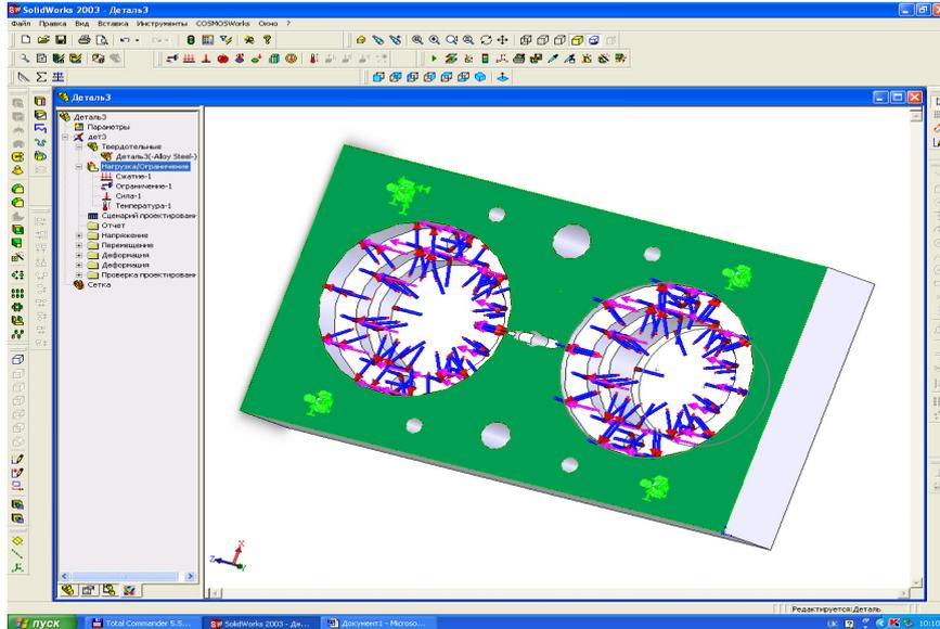
Fig. 3. The forces falling on the matrix and the fixing options
