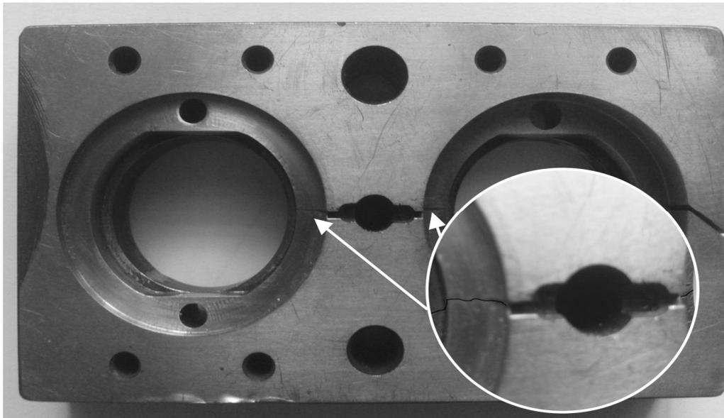
**Fig. 1.** Matrix of the press-form in which defects appeared during operation (cracks are indicated by the arrows)
