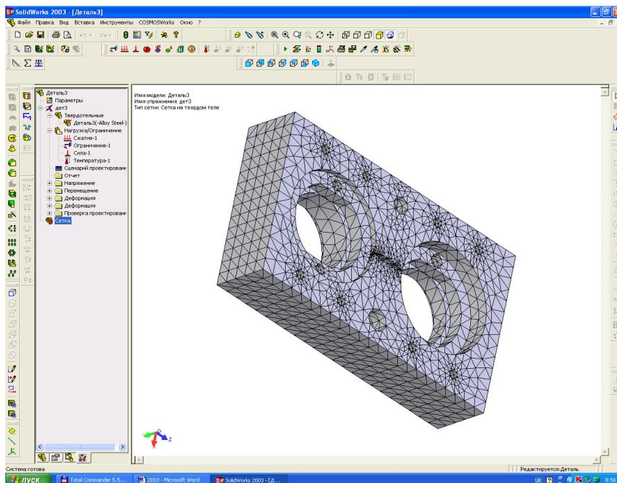
Fig. 4. Finite-element mesh
