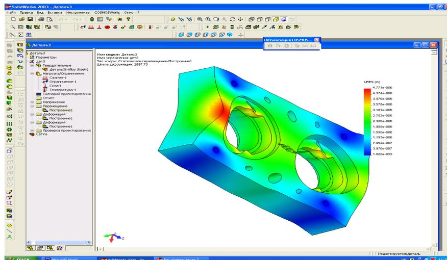
Fig. 5. Virtual results of the calculation of the deformed matrix of press-form
