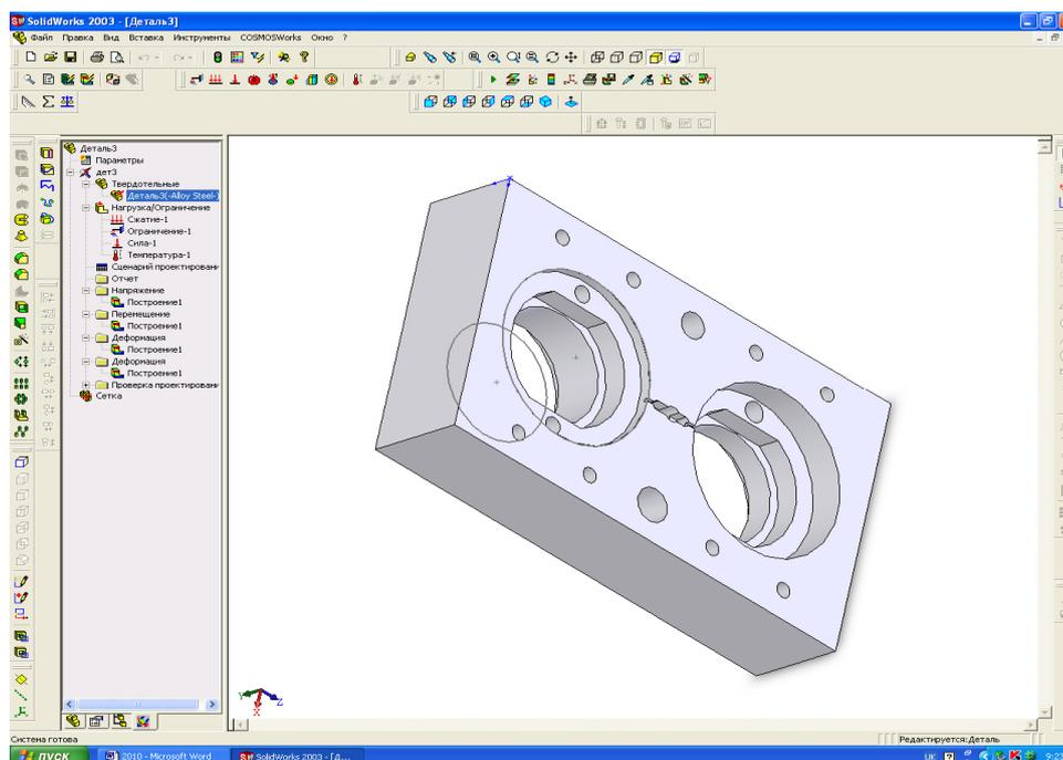
**Fig. 2.** Matrix designed in the SolidWorks system.
