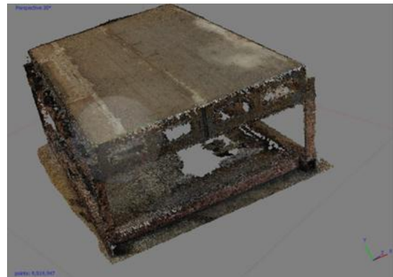
Fig. 4. Generated dense point cloud based on industrial photogrammetry results.
