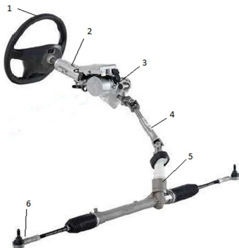
Fig. 1. Structural scheme of the electromechanical power steering: 1 – steering wheel; 2 – upper part of the steering shaft; 3 – gear motor; 4 – lower part of the steering shaft; 5 – steering rack; 6 – tip of the steering rod
