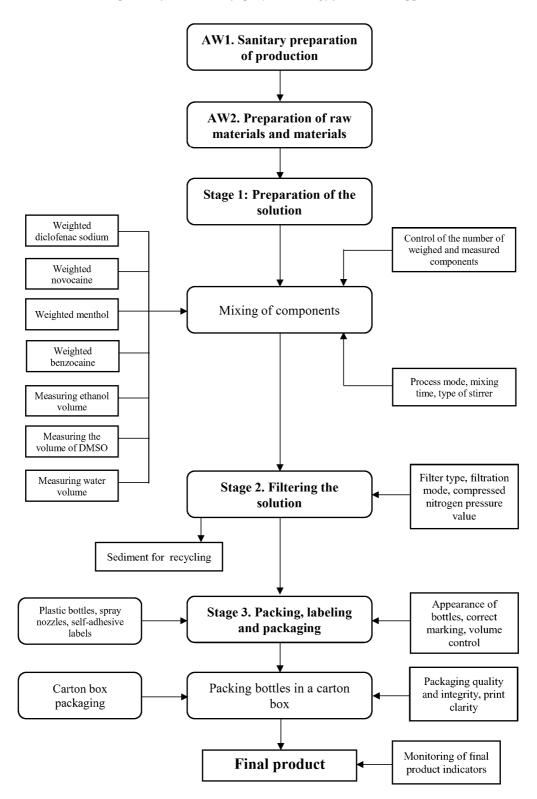
Fig. 2. Technological stages of the spray production process
