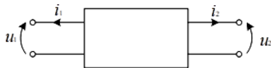
Fig. 1. Scheme of independent pole currents and polar voltages of a pass-through nonlinear active quadripole.
