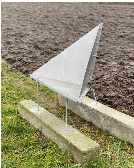
Fig. 1. Triangular corner reflector with 0.5 m inner leg length
