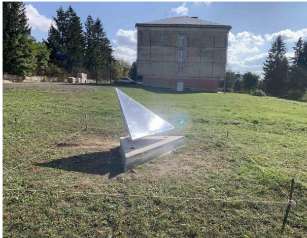
Fig. 5. Triangular corner reflector with 1.0 m inner leg length and antiflood protective screen, deployed in Berezhany
