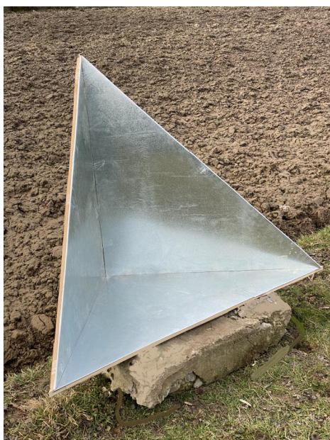
Fig. 3. Triangular corner reflector with 1.0 m inner leg length
