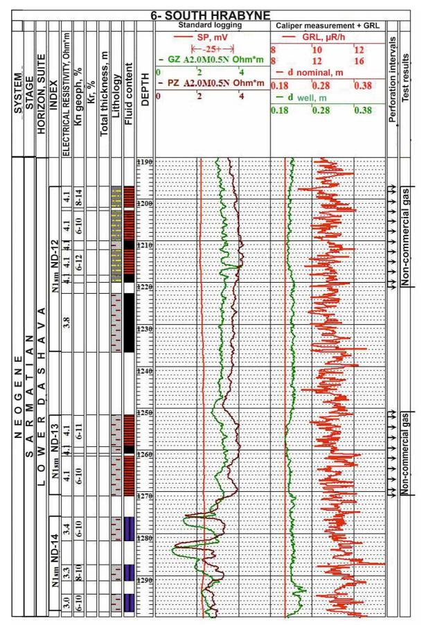
**Fig. 4.** Geological and geophysical characteristics of productive horizons ND-12, ND-13 and ND-14 in the well No. 6-South Hrabyne.
