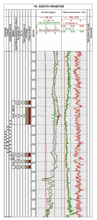
**Fig. 3.** Geological and geophysical characteristics of productive horizons ND-12 and ND-13 in the well No. 10-South Hrabyne
