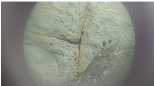
Fig. 5. A picture of the eyepiece of the optical tube aimed at the control point
