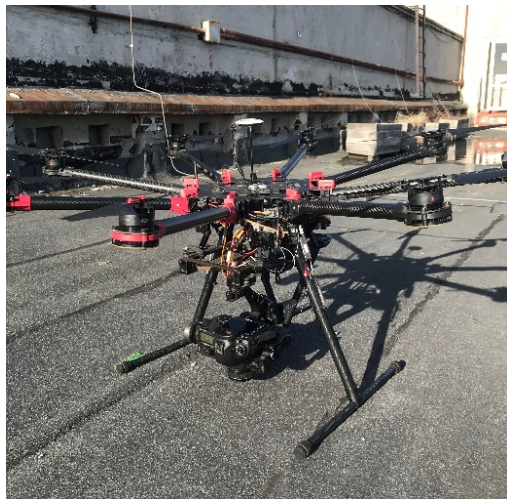
Fig. 8. General view of the octocopter DJI S1000
