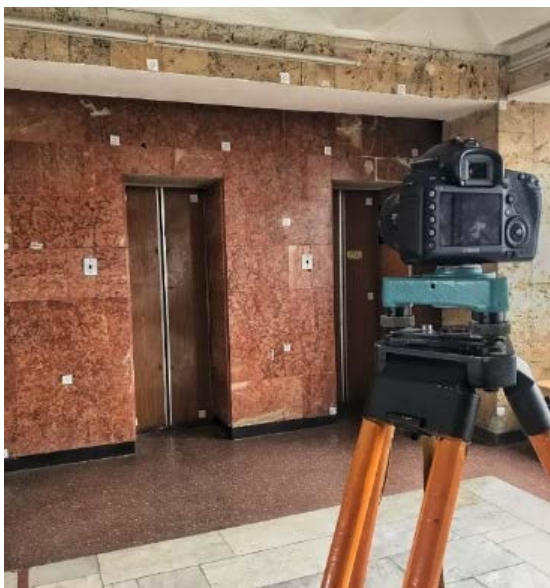
Fig. 4. Stereophotogrammetry survey of the control marks with a non-metric camera Canon EOS 5D Mark III
