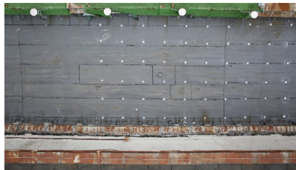
Fig. 6. The survey area with marked points which was created in the laboratory Geoterrace
