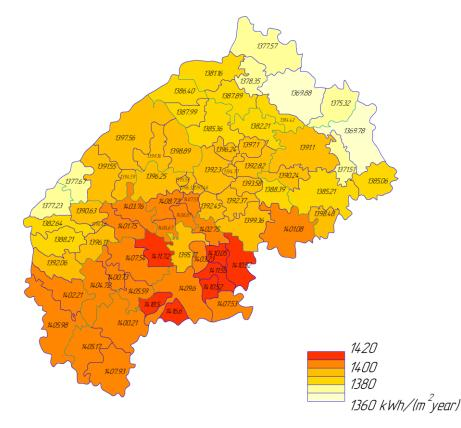
Fig.3. The annual amount of solar radiation per 1 m<sup>2</sup> of the surface, which is fixed at a fixed angle of 35°, kWh/(m<sup>2</sup> year), in the territorial communities of the Lviv region.
