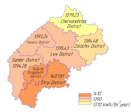
Fig.4. The annual amount of solar radiation per 1 m<sup>2</sup> of the surface, which is fixed at a fixed angle of 35°, kWh/(m<sup>2</sup> year), in the districts of Lviv region.
