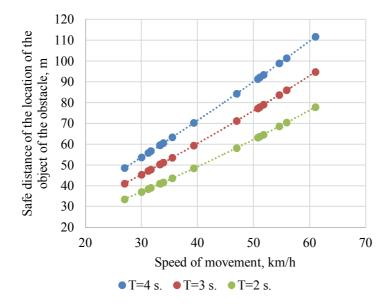
Fig. 8. Dependence of the safe distance of the location of the obstacle on the speed of movement for different values of the driver's reaction time
