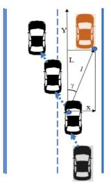
Fig. 4. The difference in the driver's subjective safety gap in the longitudinal direction of movement  $(S_d)$ and braking distance  $(S_{br})$
