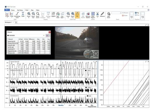
Fig. 1. Analysis window of vehicle movement parameters during interaction with an obstacle
