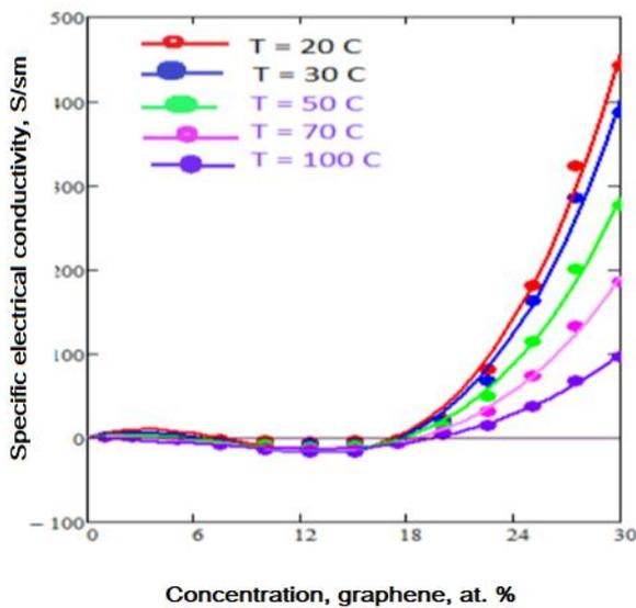
Fig. 1. Dependence of the specific electrical conductivity of Gr/PS on the concentration of graphene for different temperatures. Solid lines show the obtained functions, points correspond to the results of the experiment in [11].
