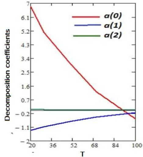
Fig. 2. Temperature dependence of decomposition coefficients obtained using the equation (1)
