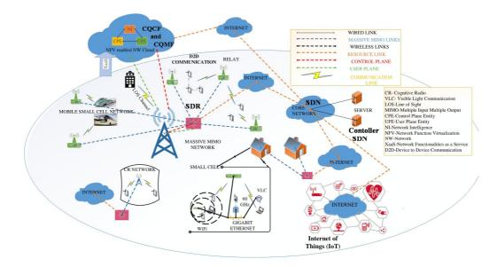
Fig. 3. The architecture of the conceptual future mobile network based on the use of SDN/SDR/NFV technologies
