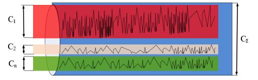
Fig. 6. Dynamic channel bandwidth allocation between three logical
