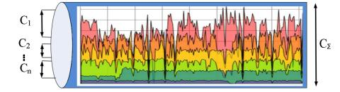
*Fig. 7. Dynamic bandwidth allocation of a physical channel between several logical channels at a certain point in time*
