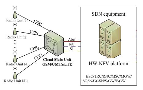
Fig. 2. Architecture of a software-defined heterogeneous mobile network
