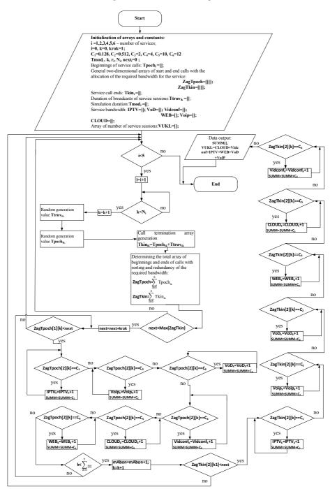
Fig. 8. Block diagram of the dynamic channel capacity allocation simulation model method
