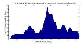
Fig. 14. The amount of bandwidth used by users when sharing a device (N = 250)
