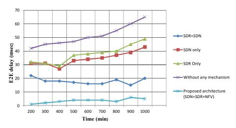
Fig. 4. Average E2E latency in the 5G-SDWN conceptual model (Software Defined Wireless Network)
