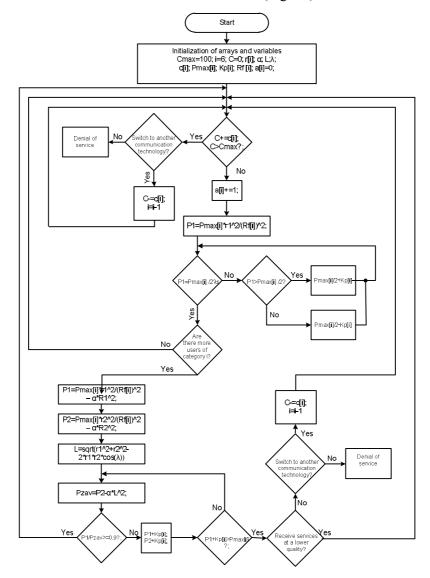
Fig. 13. Algorithm of the model for managing radio interfaces and physical resources of a femtocell
