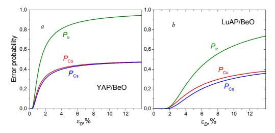
Fig. 4. Dependencies of the radioisotopes identification error probabilities  $P_{Co}$ ,  $P_{Ir}$  and  $P_{Cs}$  upon the relative error if the absorbed dose measurement  $\varepsilon_D$  according to the decision-making rule (6) and absorbed dose measurement using detectors pairs YAP/BeO (a) and LuAP/BeO (b)
