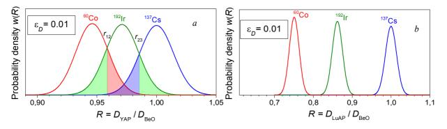
Fig. 3. The probability density distributions of estimated quantities  $R_i$  with parameters, presented in Table 2 for the detectors pairs YAP/BeO (a) and LuAP/BeO (b), in the assumption that the absorbed dose measurement possesses the Gaussian distribution of error and has a relative accuracy  $\varepsilon_D = 0.01$  (1 %)
