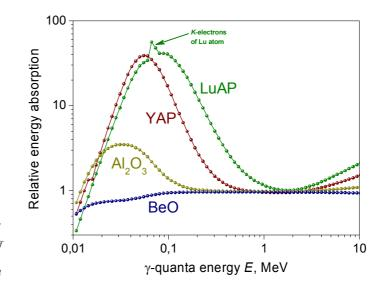
Fig. 1. Dependence of the irradiation absorption (energy deposition) upon radiation energy, obtained by Monte-Carlo simulation in [8, 18] for 1 mm thick dosimetric detectors based on BeO ( $Z_{eff}$ = 7.1), YAP ( $Z_{eff}$  = 31.4) and LuAP ( $Z_{eff}$  = 61.6), as well as  $Al_2O_3$  ( $Z_{eff}$  = 11.1) given for comparison
