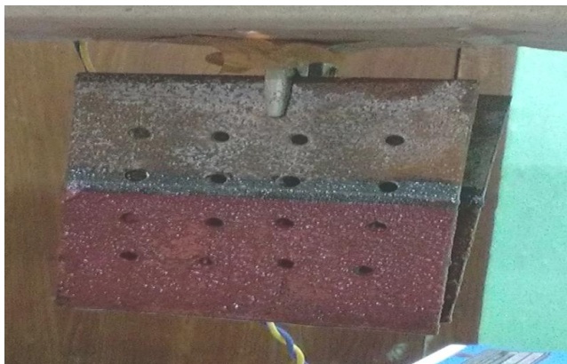
Fig. 3. Iron electrode before and after electrocoagulation process
