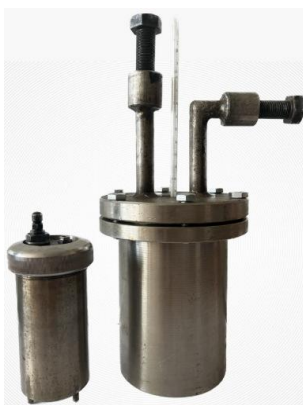
Fig. 1. View of reactors for modification of tar or bitumen with formaldehyde without stirring
