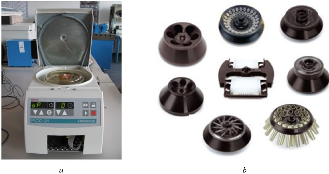
Fig. 1. Laboratory centrifuge with rotor: a – Pico 21 centrifuge; b – different rotor configurations
