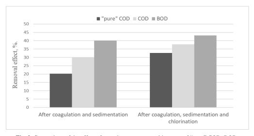
**Fig. 2.** Comparison of the effect of organic matter removal in terms of "pure" COD, BOD<sub>5</sub> and COD after coagulation and after coagulation and chlorination
