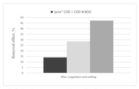
**Fig. 4.** Effect of organic matter removal in terms of "pure" COD, BOD<sub>5</sub> and COD after coagulation and settling of industrial wastewater
