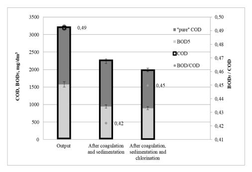
Fig. 1. Dynamics of organic matter concentration by COD, BOD<sub>5</sub> and the value of the BOD<sub>5</sub>/COD ratio
