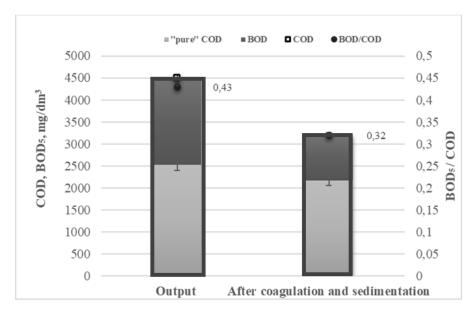
**Fig. 3.** Dynamics of organic matter concentration in terms of "pure" COD and BOD<sub>5</sub> for the initial industrial wastewater and after its coagulation
