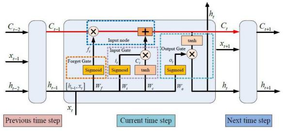
Fig. 3. LSTM principe piplines [40].
