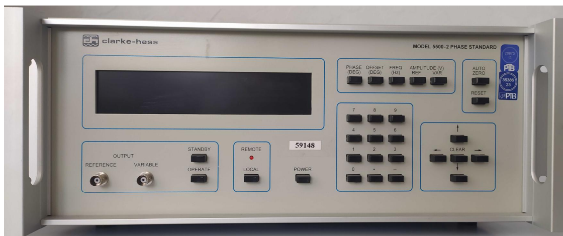
Fig. 1 General view of the phase standard Clarke-Hess 5500-2.
