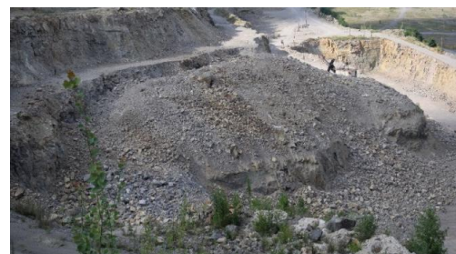
Fig. 3. Blasted rock mass removed by excavators in the Hnivanskyi quarry.
