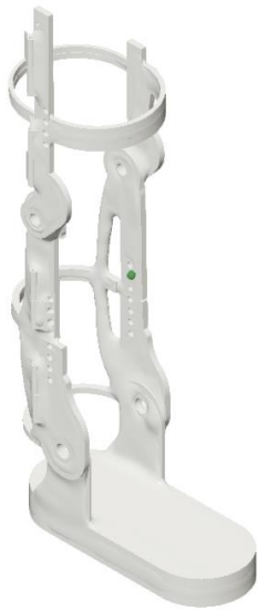
Fig. 7. The resulting 3D model of the exoskeleton after optimization.
