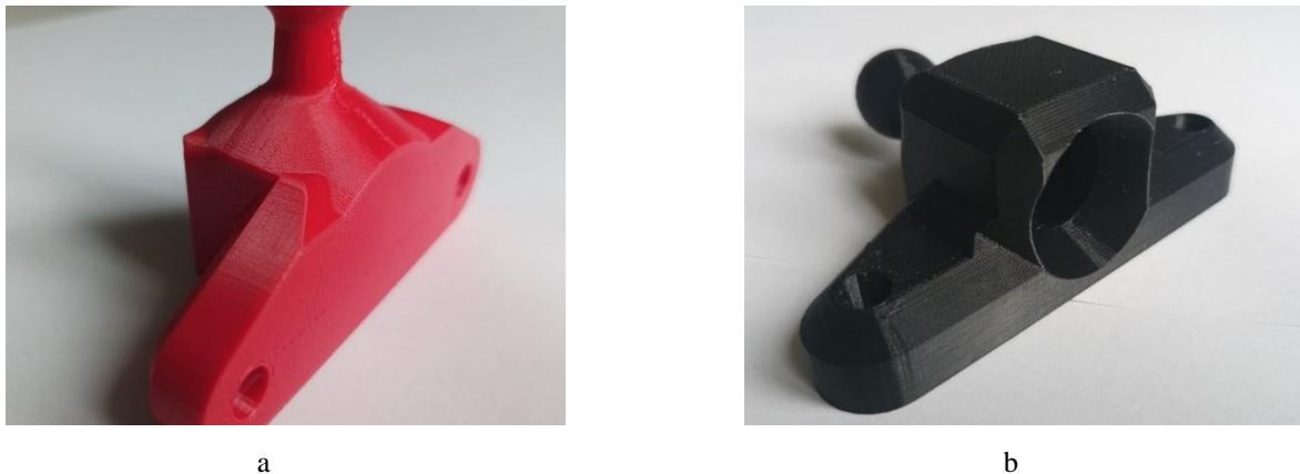
Fig. 4. The part is printed on coPET, humidity – 27 % (a); the part is printed in PLA, humidity – 33 % (b)
