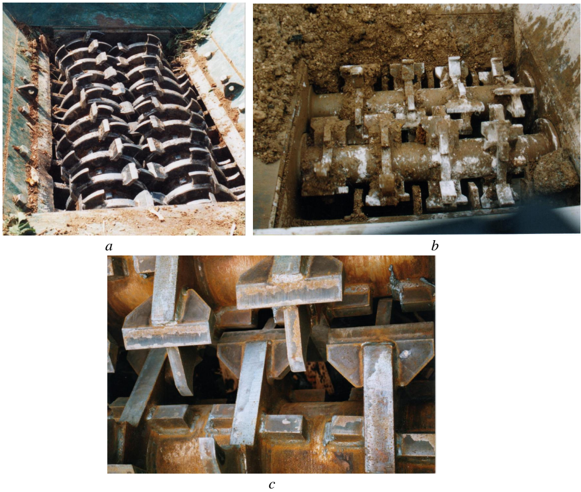
Fig. 2. The design of a shredder for processing biowaste (a), wood (b), and railway sleepers (c) by Hammel (Germany)
