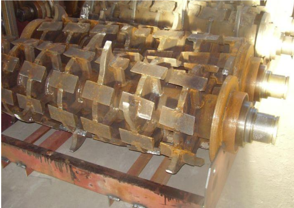
Fig. 1. Design of a 2-roll shredder by Arjes (Germany) designed for wood waste processing
