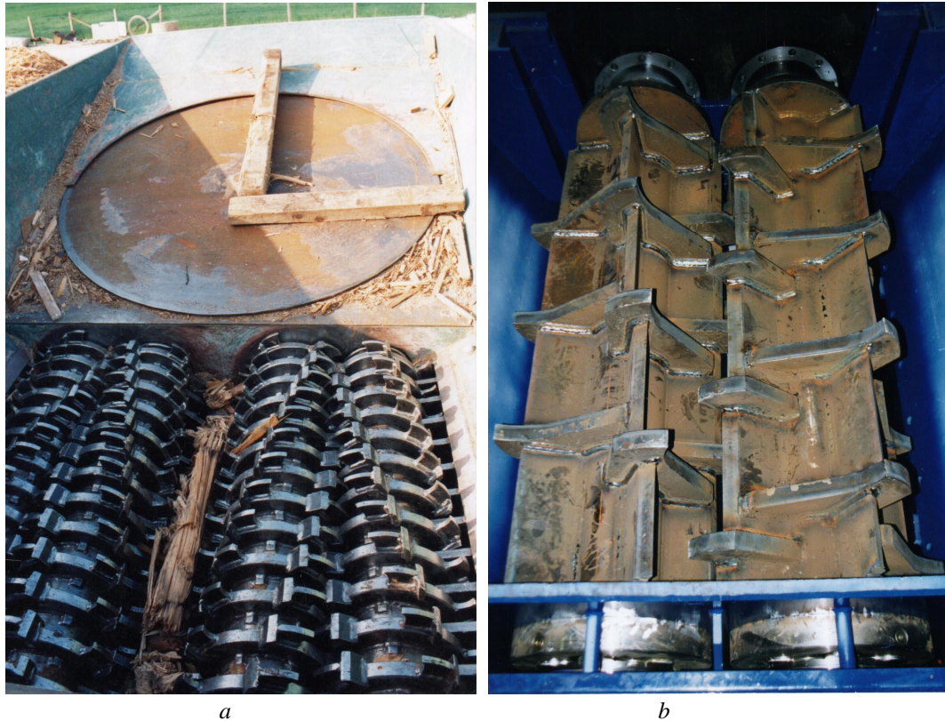
Fig. 4. Designs of 2-shaft shredders by the Pronar company (Poland), designed for processing wood and construction waste
