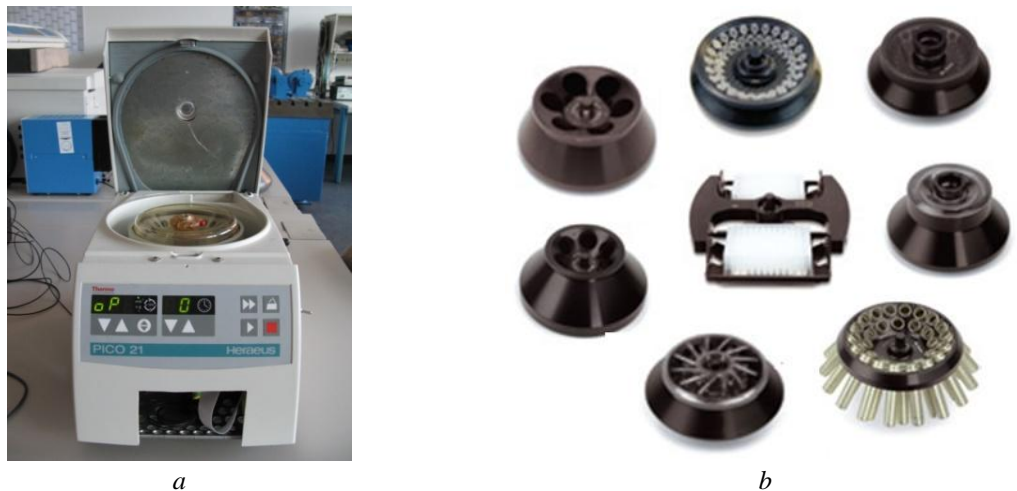
Fig. 1. Laboratory centrifuge with rotor: a – Pico 21 centrifuge; b – different rotor configurations
