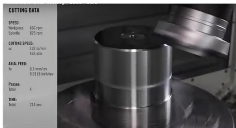
Fig. 1. Illustrates the process of cutting an external gear in the factory [2]
