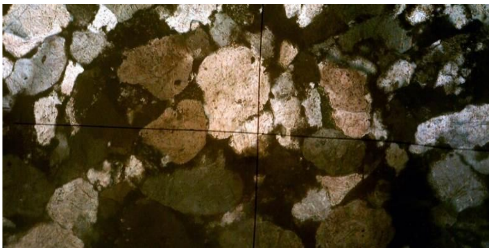
Fig. 3. The Yamna Formation. Sandstone is multi-grained, poorly sorted, siltstone with gravel, coarsely polymict, and gray. Quartz (up to 50% of the mass of the fragments), glauconite (10–15%), and lithoids (15–20%) prevail in the composition of the detrital material. Clay-silica cement with chlorite, type of cementation is porous. Photo of the cut. Nick. \times Incr. 136 x . Photo by O. Kostyuk
