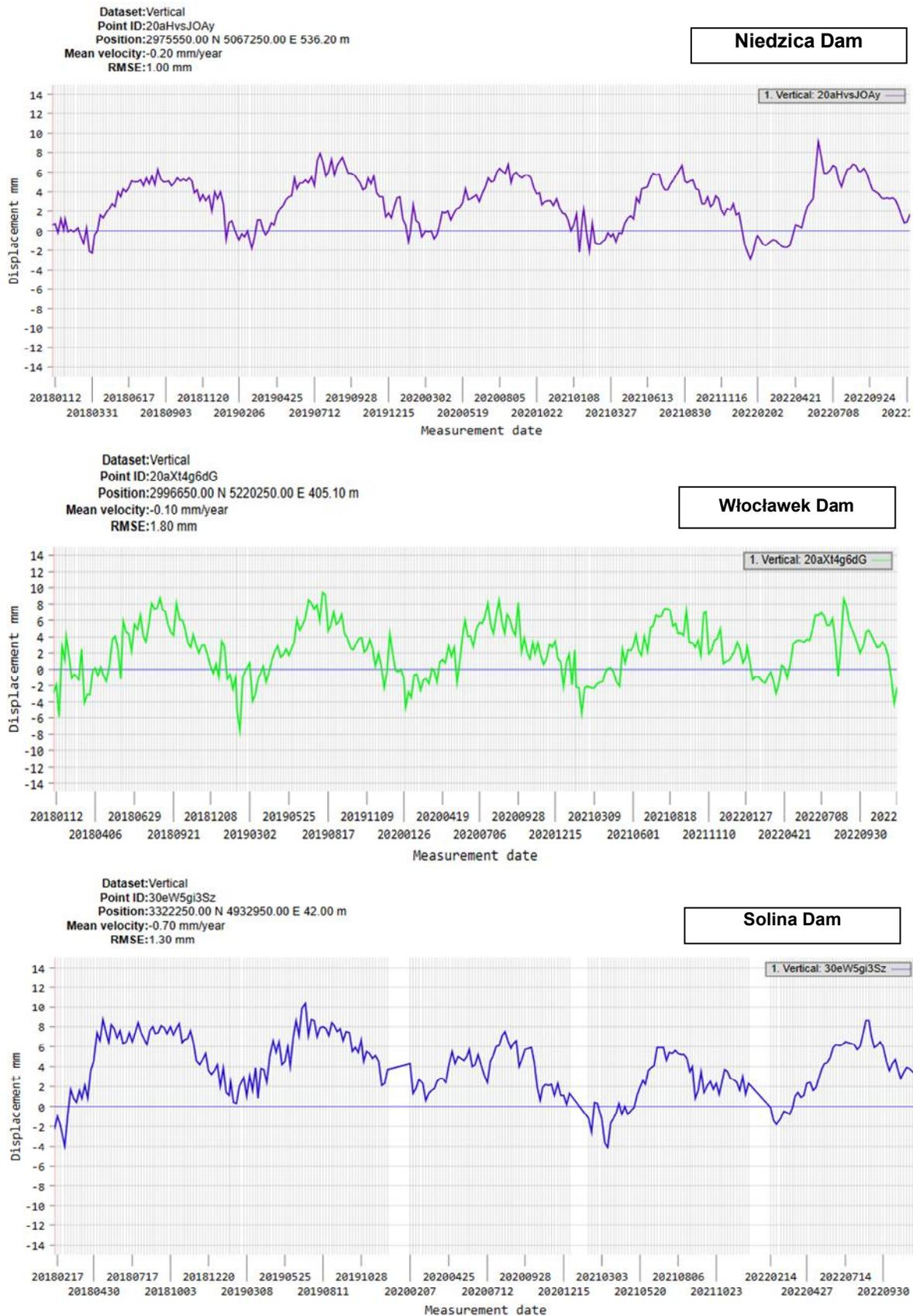
Fig. 8. Time series of vertical movements of dams: Niedzica Dam, Solina Dam, Włocławek Dam (according to EGMS)
