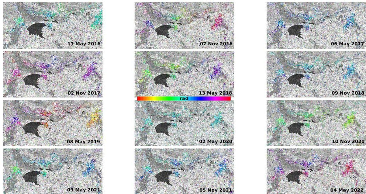
Fig. 2. Complex interferograms of each pair (master-secondary) of images. The date on the interferogram corresponds to the date of the secondary image. The phase range on the wrapped interferogram is  $[-3.14; +3.14]$
