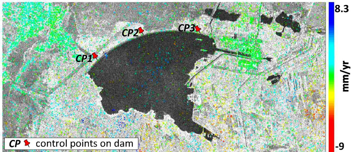
Fig. 5. Mean deformation velocity map considering spatially correlated corrections for the study area. The deformation history of the control points on the dam has been obtained from time-series analysis by the InSAR method.
