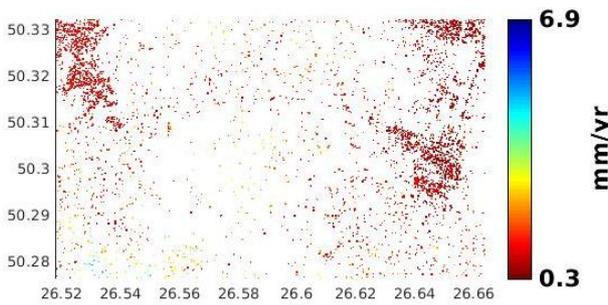
Fig. 4. Standard deviation of mean LOS velocity for the study area does not exceed 1 mm/year
