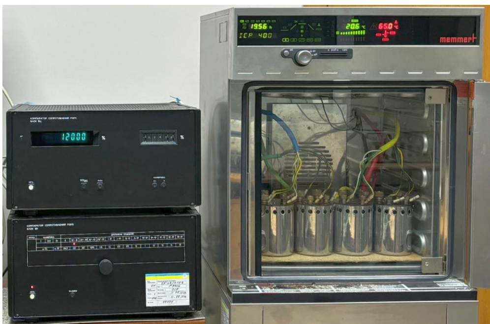
Fig. 1 The general view of the precision measurement setup for the calibration of RL
