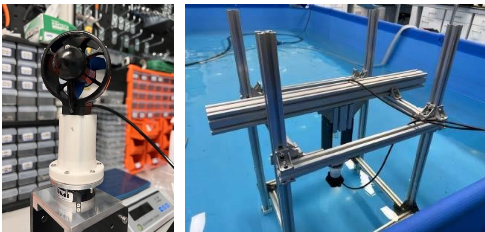
Fig. 3. Direct coupling relationship between thrusters and sensors
