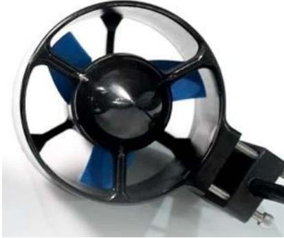
Fig. 1. Using propellers manufactured by ROVMAKER, voltage supply range: 3s-6s, maximum passing current 15A, waterproof to a depth of 300 m underwater surface
