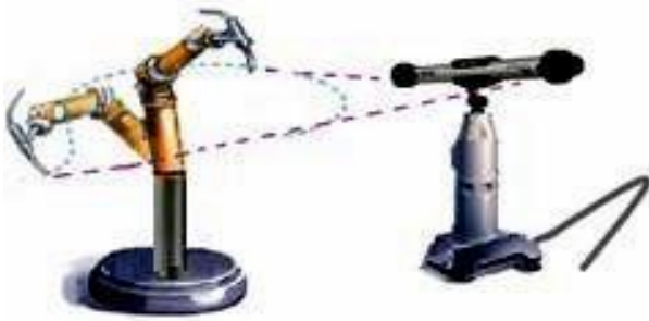
Calibration setup based on a coordinate measuring machine
